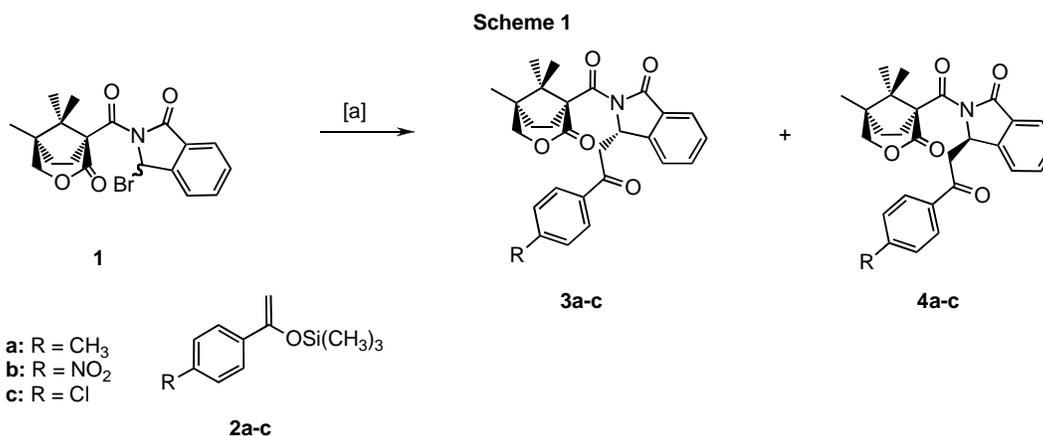
[a] Lewis acid (0.1 or 1.1 equiv.), **2a-c** (1.5 equiv.), CH<sub>2</sub>Cl<sub>2</sub>
